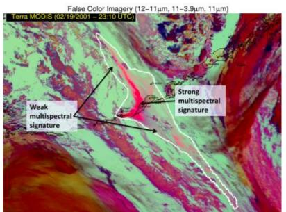
The Spectrally Enhanced Cloud Objects (SECO) algorithm is designed to identify volcanic ash and dust in manner that is more consistent with human expert interpretation of multispectral satellite imagery than traditional techniques. In an image with varying degrees of the spectral signature relative to the ash, the human eye can pick out even the faintest spectral areas and can recognize complex spatial patterns and associate that with the correct feature. The SECO method uses several advanced
