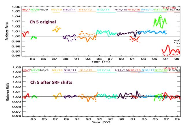
The figures above show the radiance ratios for the HIRS channel 5 for NOAA-6 through NOAA-19 and MetOp-A (M2) over a period ranging from 1982 to 2009. Prior to the correction (top panel) the ratios varied widely. After the shifts were applied (bottom panel) there was a significant reduction in the ratio differences. Ratios within .01 imply brightness temperature agreement within 0.5 K.
