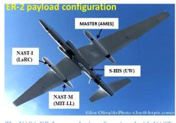
The NASA ER-2 research aircraft equipped with NAST-I, NAST-M, S-HIS and MASTER
