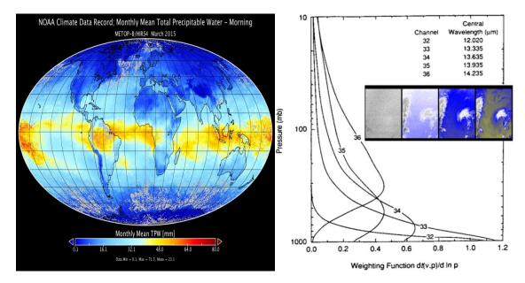
Figure: (left) Total Column Precipitable Water Vapor determined by HIRS on MetOp-A for March 2015. (right) CO2 channel weighting or contribution functions demonstrating that less opaque channels see deeper into the atmosphere, and finally to the earth surface.
