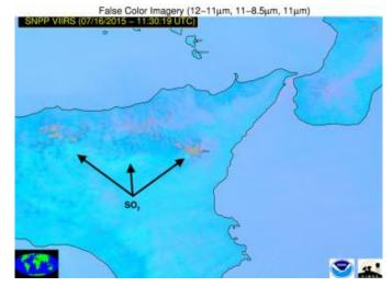
VIIRS instrument which provides high spatial resolution imagery of SO<sub>2</sub> clouds and plumes under many conditions day and night. VIIRS however has a much larger lower limit of detection compared to UV and hyperspectral IR, especially in the presence of clouds. With only one SO<sub>2</sub> absorption band, it is more challenging to extract quantitative information with VIIRS; therefore it needs to be combined with other measurements to help constrain the problem.
