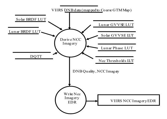
Figure 3.1.2-1. Generate NCC VIIRS Imagery EDR Level 2 Data Flow Diagram
