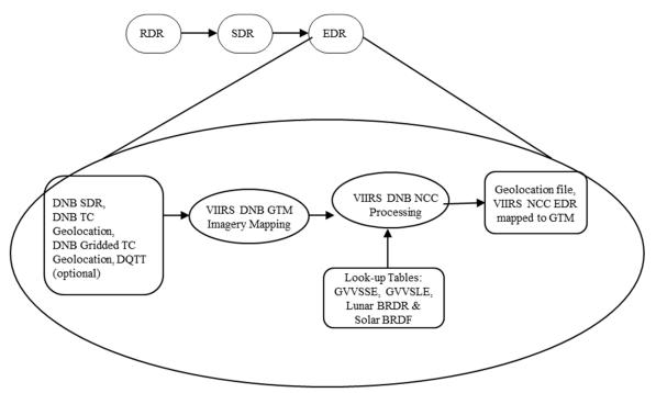
Figure 3-1. Processing Chain Associated with VIIRS NCC Imagery EDR
